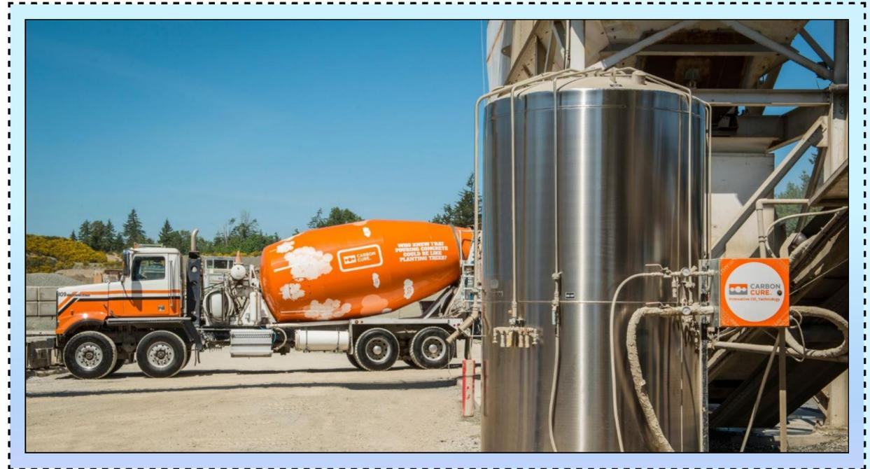
*CarbonCure's* technologies inject captured carbon dioxide into concrete, delivering the same high-quality concrete with a lower carbon footprint.
